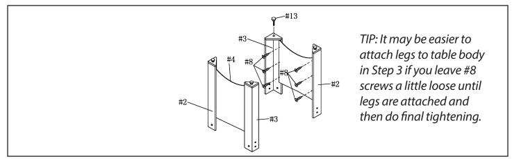
3. Attach assembled LEGS to TABLE BODY #1 with BOLT #6 and FLAT WASHER #7. Note: The table is assembled upside down.
